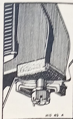
Fig. 5. This illustration shows the assembly of one of the two radiator supporting points.
