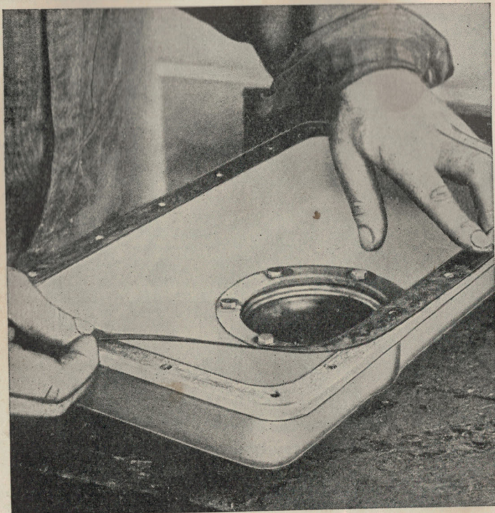
FIG. 24. THE OIL RESERVOIR OR SUMP, SHOWING A NEW JOINT WASHER BEING FITTED
