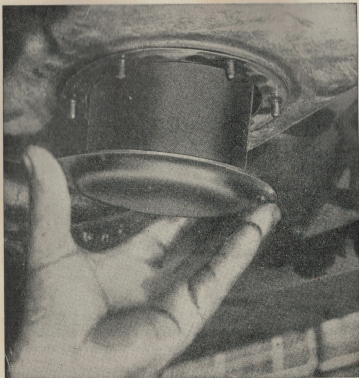
FIG. 20. REMOVING THE OIL FILTER FOR CLEANING
