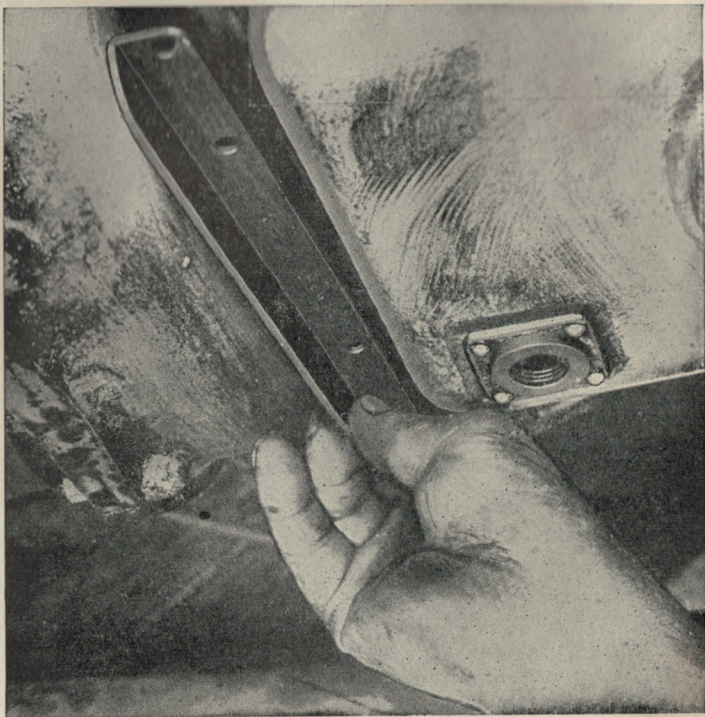
FIG. 22. THIS ANGLE STIFFENING PIECE MUST BE DETACHED BEFORE THE SUMP CAN BE REMOVED ON EARLIER MODELS
